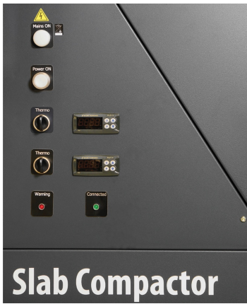
Detail of the control panel for controlling the temperature of sector head and base heating system
