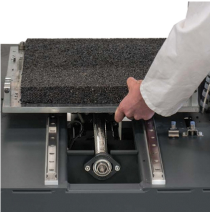
500 x 400 mm slab and lead rolled ball screw system
